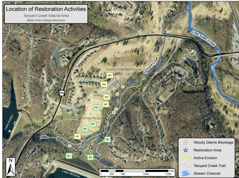
Figure 2 Identified problem areas along Tanyard Creek.
